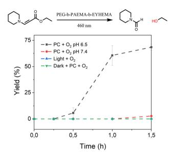
Fig. 4 The controlled activation kinetic profile of the prodrug model compound ethyl (E)-3-(piperidin-1-yl)acrylate obtained using PEG<sub>113</sub>-b-PAEMA<sub>50</sub>-EYHEMA<sub>1</sub> polymeric photocatalyst (PC, 2.5 mol%) solution in phosphate buffer solution at pH 6.5 (black) and NP-AEMA-EY in PBS buffer at pH 7.4 (red). Control reactions: without a photocatalyst in light (green) and with a photocatalyst in the dark (blue).
