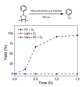
**Fig. 3** Prodrug model compound, phenylboronic acid pinacol ester, activation kinetic profiles obtained using  $PEG_{113}$ -b-PAEMA $^+_{50}$ -EYHEMA $_1$  polymeric photocatalyst (PC, 2.5 mol%) solution in phosphate buffer solution at pH 6.5 (black). Control reactions: without a photocatalyst under light (green) and with a photocatalyst in the dark (blue).
