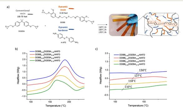
Fig. 6 (a) Synthesis of DDBB<sub>x</sub>DGEBA<sub>y</sub>/4AFD-based epoxy vitrimers (b) DSC thermograms obtained at a heating rate of 10 °C min<sup>-1</sup> for DDBB<sub>x</sub>DGEBA<sub>y</sub>/4AFD mixtures (c) corresponding  $T_g$  obtained during a second heating ramp at 10 °C min<sup>-1</sup>.
