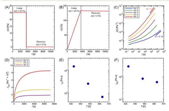
Fig. 8 Commercial polystyrene creep and recovery measurement. (A) Applied stress and (B) measured strain profiles during creep and recovery. (C) Creep and (D) recoverable compliance versus time. (E) Zero-shear viscosity and (F) steady-state relaxation time versus temperature.
