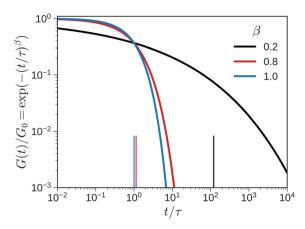
Fig. 17 The stretched exponential function for three different values of the stretching parameter.  $\beta=1$  (blue line) corresponds to  $\mathrm{e}^{-t/\tau}$ . The vertical lines on the horizontal axis mark the terminal relaxation time,  $\tau_{\mathrm{term}}^{(1)}$ , for different  $\beta$ .
