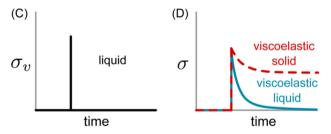
Fig. 2 (A) Applied strain profile and resulting shear stress for (B) ideal elastic solid, (C) ideal viscous liquid, and (D) viscoelastic samples.
