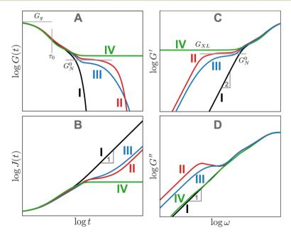
Fig. 13 Schematic for the (A) stress relaxation modulus, (B) creep compliance, (C) storage and (D) loss moduli of typical polymeric systems: (I) unentangled melt, (III) entangled melt, (III) polydisperse melt, and (IV) permanently cross-linked rubber.
