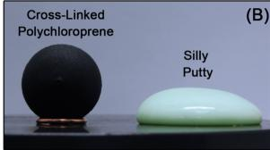
Fig. 3 Spherical samples of permanently cross-linked polychloroprene (viscoelastic solid) and silly putty (viscoelastic liquid) during annealing at 50 °C. (A) t = 0 min and (B) t = 30 min.
