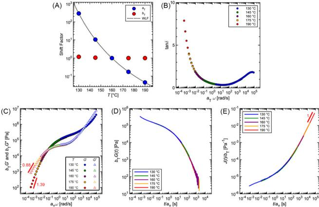
Fig. 12 Commercial polystyrene time-temperature superposition using  $T_{\text{ref}} = 160 \, ^{\circ}\text{C}$ . (A)  $a_{\text{T}}$  and  $b_{\text{T}}$  shift factors. The WLF equation is fit to the experimental  $a_T$  values. (B)  $\tan \delta$ , (C) G' and G'' (D) G(t), and (E) J(t) master curves.
