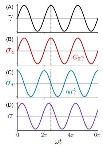
Fig. 9 SAOS waveforms. (A) Applied strain, (B) solid, (C) liquid, and (D) viscoelastic measured shear stresses.
