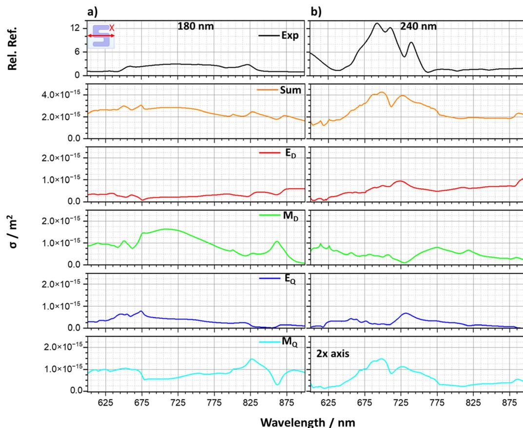
**Fig. 7** A comparison between the experimental reflectance and the total scattering cross section (and individual contributions) for a RH structure at (a) 180 nm and (b) 240 nm thickness, under  $x$ -polarised LPL. Note the increased scale of the 240 nm  $M_Q$  data.
