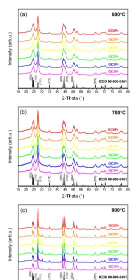
Fig. 3 XRD patterns for the series of the fabricated sol-gel samples at: 500 °C (a), 700 °C (b), and 900 °C (c).
