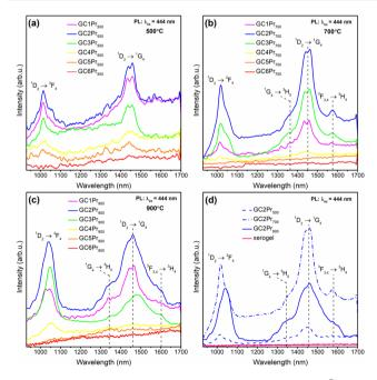
Fig. 12 Emission spectra recorded within the NIR range for Pr<sup>3+</sup>-doped sol-gel samples prepared at 500 °C (a), 700 °C (b), and 900 °C (c). The comparison of emission spectra for the as-prepared xerogels and GC2Pr<sub>x</sub> nano-glass-ceramics with La<sup>3+</sup>: Pr<sup>3+</sup> molar ratio equal to 0.994: 0.006 is also presented (d).
