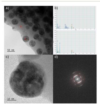
Fig. 5 TEM observations of the GC6Pr<sub>900</sub> nano-glass-ceramic sample: enlargement of the edge region showing the nanocrystals and the amorphous host regions (a) with red circles, which indicate the area used in the EDS analysis (b). HR-TEM image of the nanocrystals with visible interatomic planes (c) and corresponding FFT with the theoretical lattice distances marked by red rings (d) are also presented.
