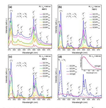
**Fig. 7** Emission spectra recorded within the VIS range for  $Pr^{3+}$ -doped sol-gel samples prepared at: 500 °C (a), 700 °C (b), and 900 °C (c). The comparison of the emission spectra for the as-prepared xerogels and  $GC2Pr_x$  nano-glass-ceramics with  $La^{3+}:Pr^{3+}$  molar ratio equal 0.994:0.006 (d); the inset in Fig. 5d shows an enlargement of the PL spectra recorded for the as-prepared xerogels.
