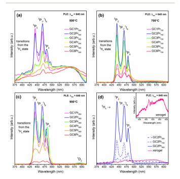
Fig. 6 Excitation spectra recorded for Pr<sup>3+</sup>-doped sol-gel nano-glassceramics fabricated at: 500 °C (a), 700 °C (b), and 900 °C (c). The comparison of excitation spectra for the as-prepared xerogels and GC2Pr<sub>x</sub> nano-glass-ceramics with La<sup>3+</sup>: Pr<sup>3+</sup> molar ratio equal 0.994: 0.006 (d); the inset in (d) shows an enlargement of the PLE spectra recorded for the as-prepared xerogels.
