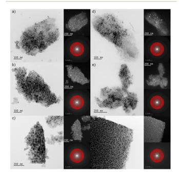
Fig. 4 TEM observations of the GC1Pr, (left side) and GC6Pr, (right side) for the nano-glass-ceramics obtained during heat-treatment at 500 °C (a and b), 700 °C (c and d), and 900 °C (e and f). The right part of the columns presents corresponding dark field images and recorded SAED patterns. Red circles indicate theoretical Bragg positions.
