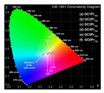
Fig. 10 CIE chromaticity diagram with coordinates assigned for Pr<sup>3+</sup>-doped nano-glass-ceramics prepared at 700 °C.
