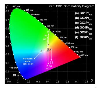
Fig. 11 CIE chromaticity diagram with coordinates assigned for Pr<sup>3+</sup>doped nano-glass-ceramics prepared at 900 °C.
