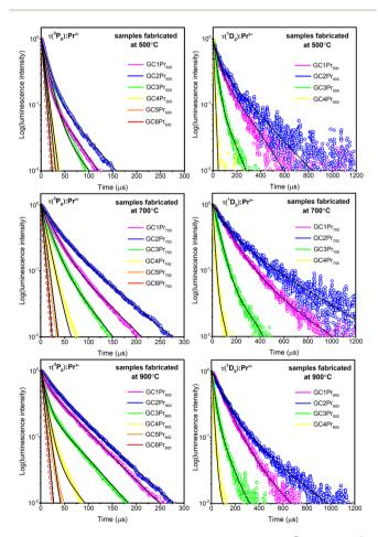
Fig. 13 Luminescence decay curves recorded for the <sup>3</sup>P<sub>0</sub> and the <sup>1</sup>D<sub>2</sub> states of Pr3+ ions in the fabricated nano-glass-ceramic samples.
