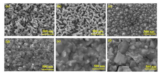
Fig. 1 FESEM image of (a)  $BiVO_4$ , (b)  $BiVO_4$ /NiOOH/FeOOH nanostructured photoanodes, (c) pure  $Cu_2O$ , (d)  $Cu_2O$ /CuO, (e)  $Cu_2O$ /CuO/ $TiO_2$  and (f) CuO photocathode.
