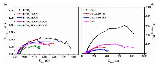
Fig. 6 Electrochemical impedance spectra (EIS) of (a)  $BiVO_4$ /FeOOH,  $BiVO_4$ /NiOOH,  $BiVO_4$ /FeOOH/NiOOH and  $BiVO_4$ /NiOOH/FeOOH photoanodes and (b)  $Cu_2O$ ,  $Cu_2O$ /CuO,  $Cu_2O$ /CuO/CuO/CuO/CuO) photocathodes tested in 0.1 M  $Na_2SO_4$  (pH 6) in AM 1.5 G equipped illumination source with a power intensity of 100 mW cm $^{-2}$ .
