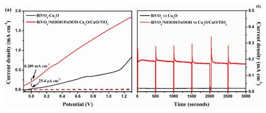
Fig. 9 (a) Two-electrode LSV responses, (b) stability tests (j vs. t) of BiVO<sub>4</sub> vs. Cu<sub>2</sub>O and BiVO<sub>4</sub>/FeOOH/NiOOH vs. Cu<sub>2</sub>O/CuO/TiO<sub>2</sub> tandem cell tested in 0.1 M Na<sub>2</sub>SO<sub>4</sub> (pH 6) in AM 1.5 G equipped illumination source with a power intensity of 100 mW cm<sup>-2</sup>. The chopping of light was carried out every 500 seconds.
