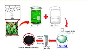
Fig. 6 Green reduction of graphene oxide (GO) using an aqueous leaves extract.
