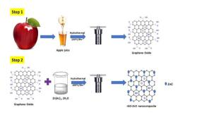
Synthesis of GO and rGO/ZnO NCs via hydrothermal method.
