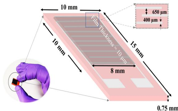
Fig. 3 Thin film-based sensor fabrication over IDE.
