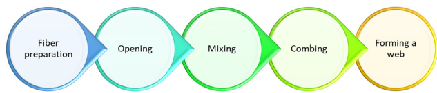
Fig. 3 Steps involved in the formation of nonwovens.
