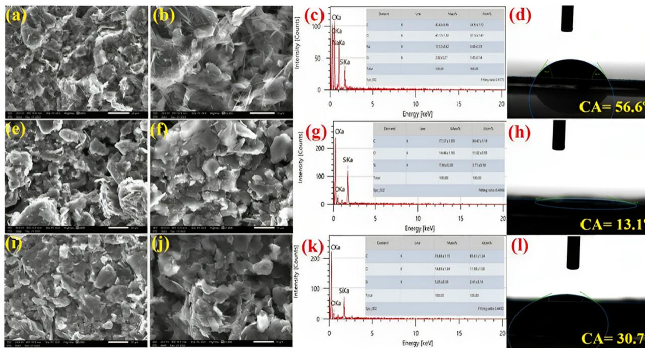
Fig. 3 SEM images of the SPE at (a) low (20  $\mu\text{m}$ ) and (b) high (10  $\mu\text{m}$ ) magnification; (c) EDS, and (d) CA. SEM images of anti-CYFRA21-1/SPE at (e) low (20  $\mu\text{m}$ ) and (f) high (10  $\mu\text{m}$ ) magnifications; (g) EDS and (h) CA. SEM images of anti-TP53/SPE at (i) low (20  $\mu\text{m}$ ) and (j) high (10  $\mu\text{m}$ ) magnifications; (k) EDS and (l) CA.
