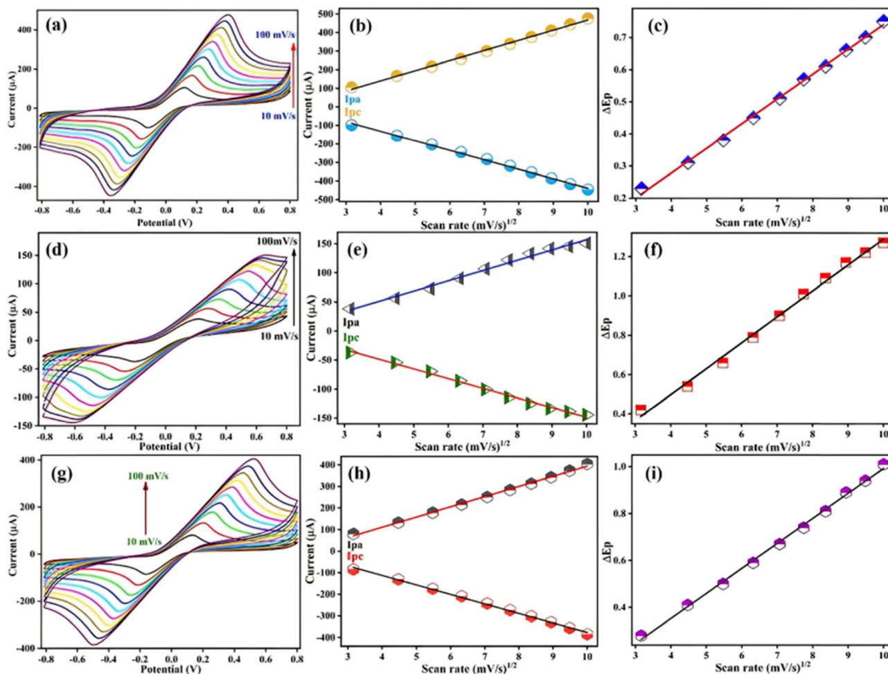
Fig. 5 Scan rate analysis of different electrodes: (a) SPE, (d) BSA/anti-CYFRA21-1/SPE, and (g) BSA/anti-TP53/SPE in PBS.  $I_{pa}$  and  $I_{pc}$  peak current curves of (b) SPE, (e) BSA CYFRA21-1/SPE and (h) BSA/anti-TP53/SPE electrodes, respectively, with the square root of scan rates. Changes in peak potential ( $\Delta E_p$ ) versus the square root of scan rates for (c) SPE, (f) BSA/CYFRA21-1/SPE and (i) BSA/anti-TP53/SPE bioelectrodes, respectively.
