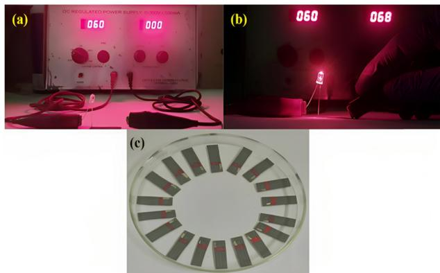
Fig. 1 The LED bulb demonstrates the (a) off-condition in an open circuit, and (b) on-condition in a closed circuit at 59 V of direct current; (c) a three-electrode disposable paper-based SPE.
