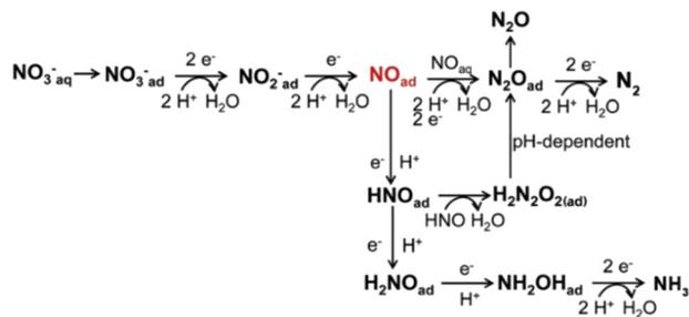
Fig. 2 Reaction pathway diagram for nitrate electroreduction.
