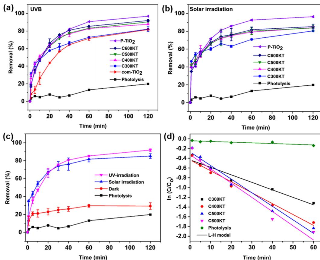
Fig. 4 Degradation of TET under (a) UVB and (b) solar irradiation using com-TiO<sub>2</sub>, P-TiO<sub>2</sub>, C300KT, C400KT, C500KT, and C600KT along with the control photolysis experiment (no catalyst present), (c) comparison of the efficiency of C600KT with the dark experiment, and (d) Langmuir-Hinshelwood kinetic fits for all measurements. Some of the error bars are small and directly on the plot symbols, the same figure only showing the error bars can be found in the Fig. S3†
