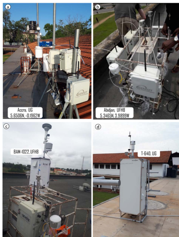
Fig. 2 Pictures of monitors, (a) RAMPs at UFHB, (b) RAMPs at UG, (c) collocation of BAM-1022 and RAMPs at UFHB, (d) Teledyne T-640 at UG.
