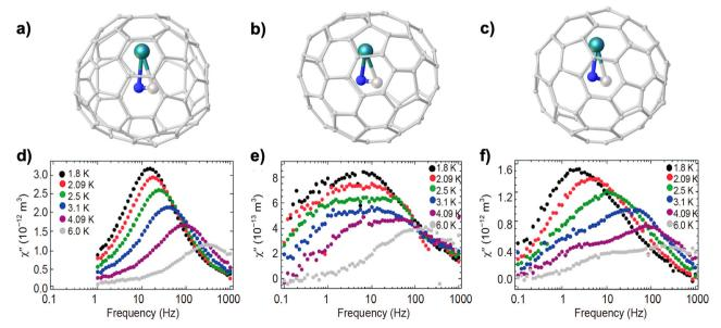
Fig. 5 Molecular structures of TbCN@ $C_2(5)$ -C<sub>82</sub> (a), TbCN@ $C_5(6)$ -C<sub>82</sub> (b) and TbCN@ $C_2(9)$ -C<sub>82</sub> (c). Out-of-phase AC magnetic susceptibility of TbCN@ $C_2$ (5)-C<sub>82</sub> (d), TbCN@ $C_s$ (6)-C<sub>82</sub> (e) and TbCN@ $C_2$ (9)-C<sub>82</sub> (f) at 1.8-6 K. Reproduced from ref. 100.
