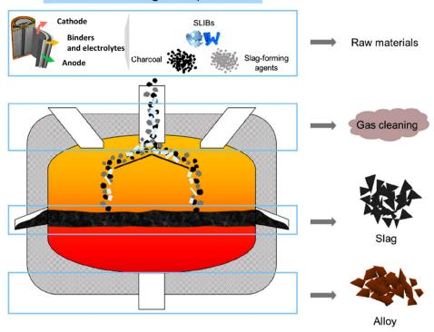
Fig. 4 Typical pyrometallurgical processes of spent LIBs. Reproduced with permission from ref. 62; Copyright 2021, American Chemical Society.
