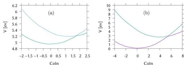
Fig. 2 Cuts through the LVC potential energy surfaces for (a) IC2 (DMABN) and (b) IC3 (fulvene) along the vector from FC to MECI. For IC2 the  $S_1/S_2$  surfaces are shown, while for IC3 the surfaces are for  $S_0/S_1$ .
