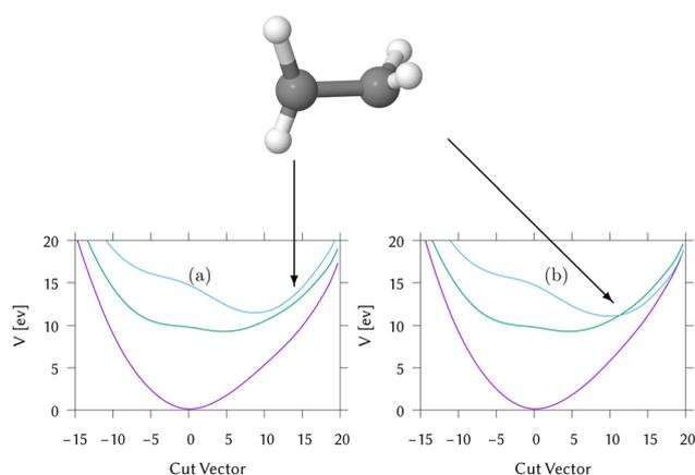
Fig. 8 Cut through the (a) adiabatic and (b) diabatic potential surfaces of IC1 from the Franck–Condon point (at a distance of 0) to a representative geometry where hopping takes place (at a distance of 13.0). The geometry is shown above the cuts.
