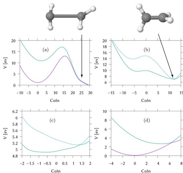
**Fig. 5** Cut through the direct dynamics potential energy surfaces from the FC point to the MECIs (a) of  $S_0/S_1$  for IC1 (ethene) (b) of  $S_1/S_2$  for IC1 (ethene) (c) of  $S_1/S_2$  for IC2 (DMABN) (d) of  $S_0/S_1$  for IC3 (fulvene). The x-axis is labelled “Coln” to emphasise that this data does not represent motion along a specific normal mode. Key: purple =  $S_0$ , green =  $S_1$ , blue =  $S_2$ .
