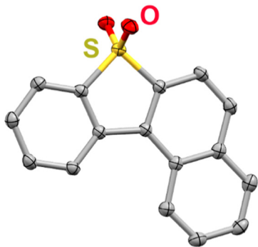
Fig. 2 Molecular structure of BNTD obtained from single-crystal X-ray diffraction studies. Yellow = S, red = O, gray = C; thermal ellipsoids at 50%; H atoms are omitted for clarity. CCDC 2350924.†
