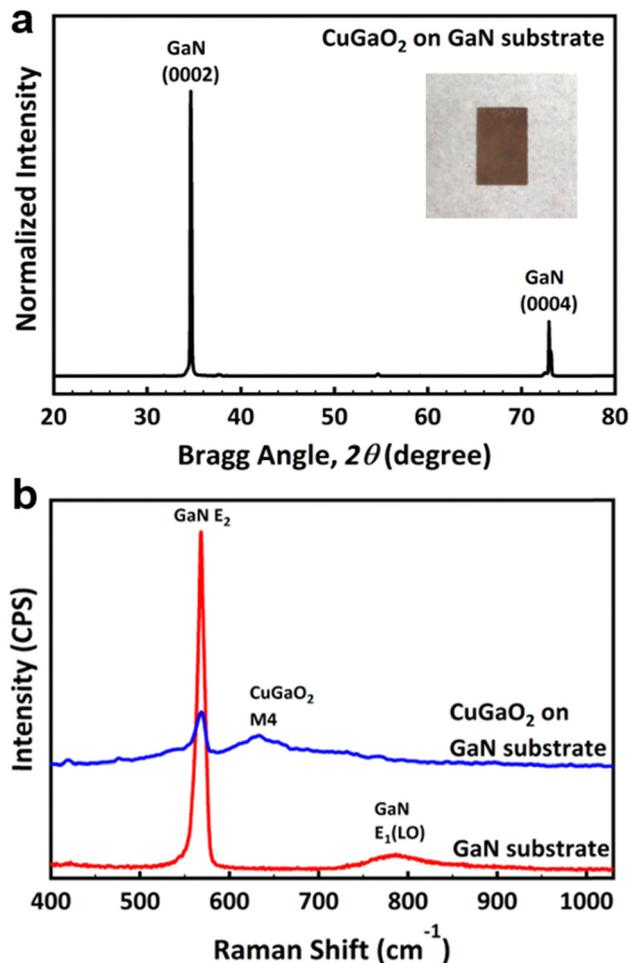
Fig. 2 (a) XRD profile of a CuGaO<sub>2</sub> film grown on the GaN substrate with a digital photograph of it in the inset, and (b) Raman spectra of the GaN substrate before and after epitaxial growth.
