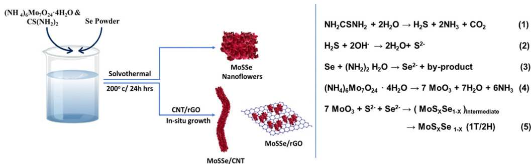
Fig. 1 A schematic illustration demonstrating the synthesis of bare MoSSe, MoSSe@CNT, and MoSSe@RGO nanocomposites via a solvothermal approach and the right panel showing the various reaction intermediates generated during MoSSe growth.
