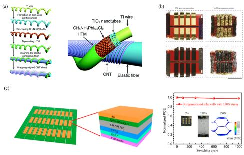
Fig. 3 (a) Schematic illustration of the elastic PSC fibre; 53 (b) schematic of the ultrathin and buckling FPSCs; 54 (c) schematic illustration of the kirigamibased PSC array and structure of PSCs and normalized PCE of kirigami-based PSCs after different stretching cycles.<sup>55</sup>
