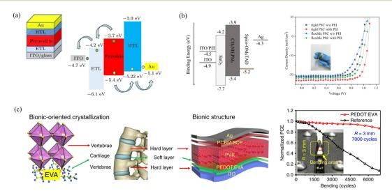
Fig. 2 (a) Structure and energy band diagram of perovskite solar cell;  $^{44}$  (b) the energy levels of the materials used in the devices and the J-V curves of the champion devices with and without PEI, 43 (c) biomimetic mechanisms of the vertebrae and PSCs and normalized averaged PCE value for the flexible PSCs under bending cycles with radius of 3 mm. 46
