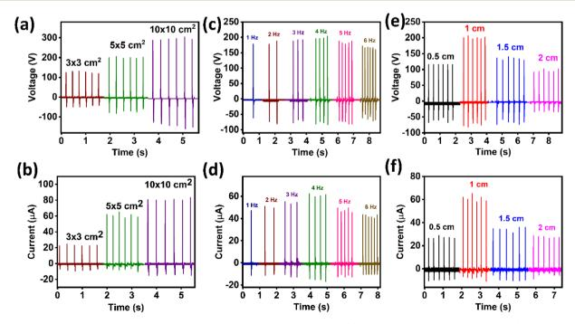
Fig. 5 Comparative study of TENG open circuit voltage and short circuit with (a) and (b) different active areas of the devices, (c) and (d) different frequencies of applied force, and (e) and (f) different spacings between the triboelectric layers
