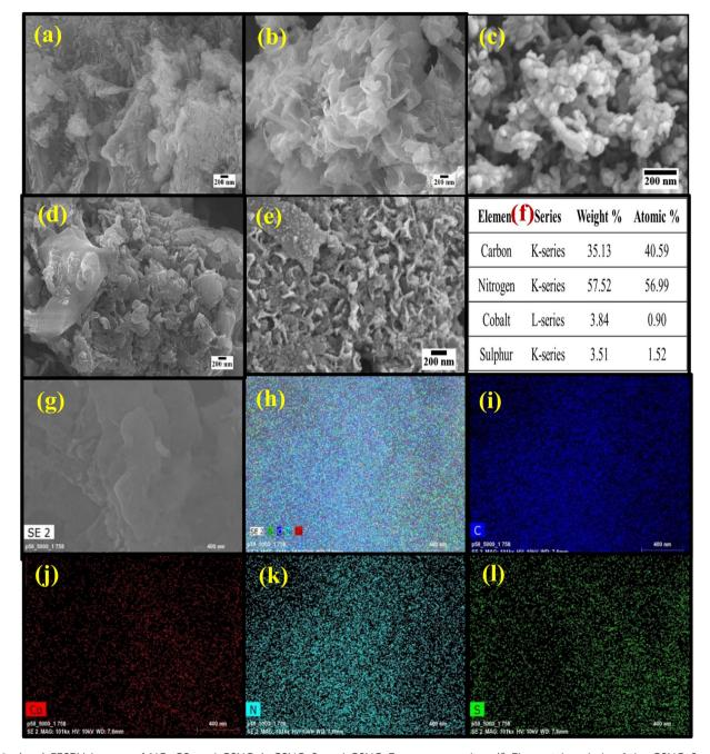
Fig. 2 (a-e) FESEM images of NG, CS, and CSNG-1, CSNG-2, and CSNG-3 nanocomposites. (f) Elemental analysis of the CSNG-2 nanocomposite. (g-l) Elemental mapping of the CSNG-2 nanocomposite.
