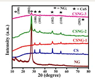
Fig. 1 XRD of NG, CS, and CSNG nanocomposites.
