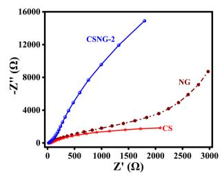
Fig. 6 EIS Nyquist plots of pure NG, CS, and the nanocomposite.
