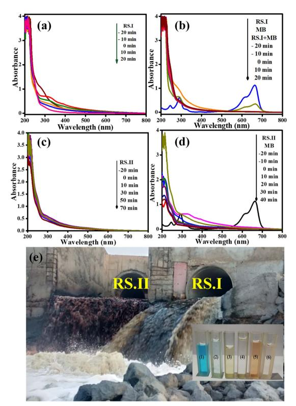
Fig. 9 (a and c) Real sample analysis using the CSNG-2 nanocomposite with RS.I and RS.II, and (b and d) real sample analysis with MB dye using the CSNG-2 nanocomposite. (e) Real sample location sites (RS.I, and RS.II); the inset shows the digital images of MB, RS.I and RS.II before and after degradation with the catalyst, respectively.
