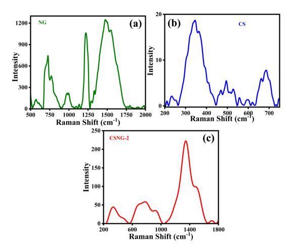
Raman spectra of (a) NG, (b) CS, and (c) CSNG-2 nanocomposite
