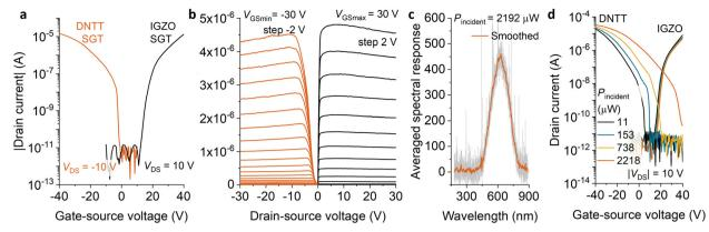
Fig. 2 (a) Transfer and (b) output characteristics for the IGZO and DNTT SGTs having channel widths  $W_{\text{DNTT}}$  = 200  $\mu$ m and  $W_{\text{IGZO}}$  = 90  $\mu$ m. Both transistors operate in enhancement mode, have large on-off current ratio and similar on-state drain currents; (c) measured spectral response of the light source used for photostimulation; (d) transfer characteristics for the IGZO and DNTT SGTs under illumination using the light source in (c) at different intensities.
