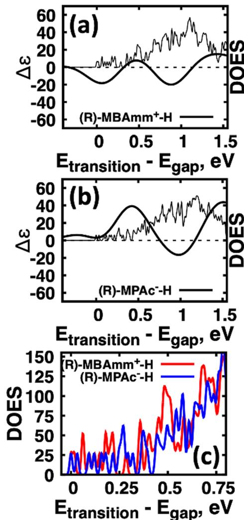
**Fig. 5** Comparison of chirality transfer for (R)-MBAm<sup>+</sup>-H and (R)-MPAc<sup>-</sup>-H. Overlay of CD spectra and DOES for (a) (R)-MBAm<sup>+</sup>-H and (b) (R)-MPAc<sup>-</sup>-H. (c) DOES overlaid for (R)-MBAm<sup>+</sup>-H (red) and (R)-MPAc<sup>-</sup>-H (blue).
