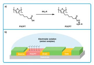
Fig. 15 P3CPT based electrolyte-gated OTFT sensor for biogenic amines. (a) Mechanism for the interaction of P3CPT polymers and amine analytes showing a deprotonation of P3CPT. (b) Cross section showing the sidegate architecture used for the fabrication of OTFT sensors. Modified with permission from Minami et al. 172
