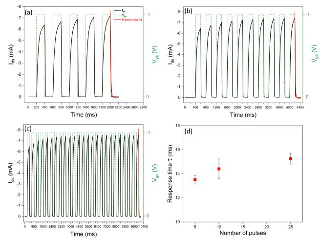
Fig. 3 Transient  $I_{\rm ds}$  response of [EMIM][TFSI]-gated P3HT transistors in response to different numbers of  $V_{\rm gs}$  square step train pulses.  $V_{\rm gs} = -1\,{\rm V}$  at  $V_{\rm ds} = -1\,{\rm V}$ -0.6 V (a) 5 pulses, (b) 10 pulses, (c) 25 pulses. (d) Response time versus number of  $V_{\rm qs}$  pulses. The duration and interval of each  $V_{\rm qs}$  pulse is 200 ms; exponential fits used to estimate the response time are in red.
