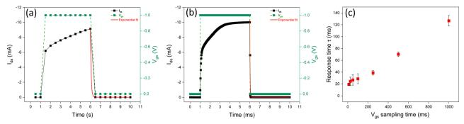
Fig. 5 Transient response of an [EMIM][TFSI]-gated P3HT transistor at different  $V_{qs}$  pulse sampling times: (a) 500 ms, (b) 25 ms; the duration of  $V_{qs}$  pulse is 5 s. (c) Response time versus different  $V_{\rm qs}$  sampling times (10, 25, 50, 100, 200, 500, and 1000 ms) at  $V_{\rm ds} = -0.8$  V.
