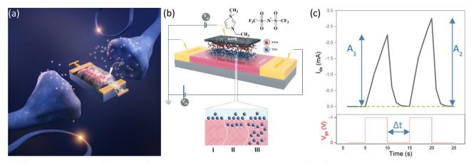
Fig. 1 (a) Bio-inspired synaptic IGT transistor. (b) Device scheme and possible doping regimes (I to III) upon application of a negative  $V_{as}$  to a P3HTbased IGT; molecular structures of the ions constituting the ionic liquid employed as gating medium in this study. (c) A pair of successive  $V_{as}$  inputs (-1 V) for 5 s with a pulse interval  $\Delta t = 5$  s applied to an IGT.  $A_1$  and  $A_2$  are the amplitudes of the drain-source current ( $I_{ds}$ )
