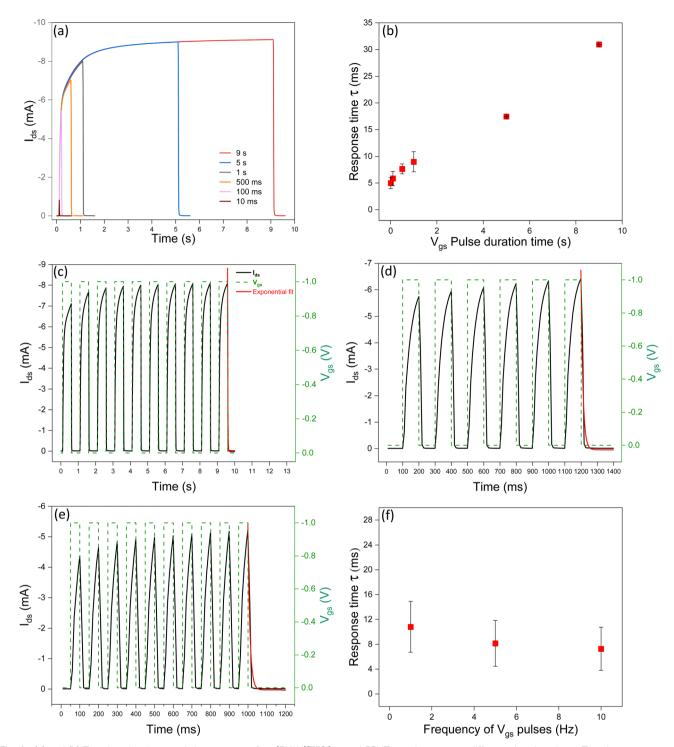
Fig. 4 (a) and (b) Transient I<sub>ds</sub> characteristic response of an [EMIM][TFSI]-gated P3HT transistor versus different duration times. Transient response of transistors in response to  $V_{qs}$  pulses with different frequencies (c) 1 Hz, (d) 5 Hz, and (e) 10 Hz. (f) Response time versus frequency of  $V_{qs}$  pulses ( $V_{qs} = -1 \text{ V}$ , at  $V_{\rm ds} = -0.6 \text{ V}$ ).
