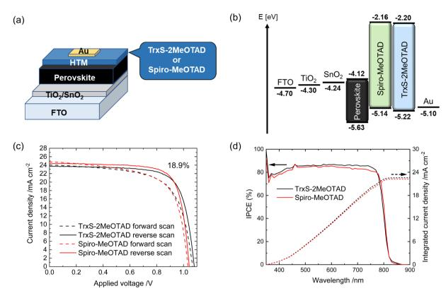
Fig. 7 (a) The PSC device structure employed in this study. (b) The corresponding energy level diagram. The values for FTO,  $TiO_2$ ,  $SnO_2$  and Au were taken from the literature. (c) J-V curves of the best TrxS-2MeOTAD PSC and spiro-MeOTAD PSC fabricated in this study. (d) The corresponding IPCE curves.
