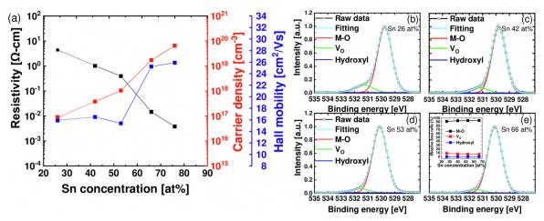
Fig. 4 (a) Resistivity, carrier density, and Hall mobility for ZTO films as a function of Sn concentration. XPS O 1s spectra and their deconvolution for the ZTO films with (b) Sn 26 at%, (c) Sn 42 at%, (d) Sn 53 at%, (e) Sn 66 at%. The inset in the panel shows the variation of the relative area ratio calculated from the O 1s spectra as a function of Sn concentration.
