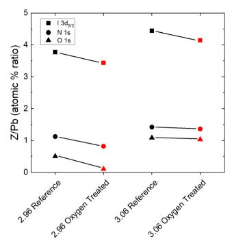
Fig. 4 The atomic percentage ratios or iodine, nitrogen, and oxygen relative to the Pb4f<sub>7/2</sub> doublet for an understoichiometric and overstoichiometric sample. All ratios decrease upon photooxgen treatment.
