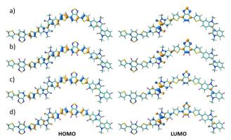
DFT-calculated HOMO (right) and LUMO (left) topologies for the dimeric models of P1 (a), P2 (b), P3 (c) and P4 (d) polymers at the B3LYP/ 6-31G\*\* level of theory
