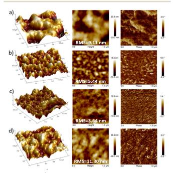
Fig. 9  $1 \times 1 \mu m^2$  tapping-mode AFM images of 3D-topography (left), height (middle) and phase (right) for (a) P1, (b) P2, (c) P3 and (d) P4 films prepared under optimal device performance conditions. The corresponding root-mean-square (RMS) roughness is also shown.
