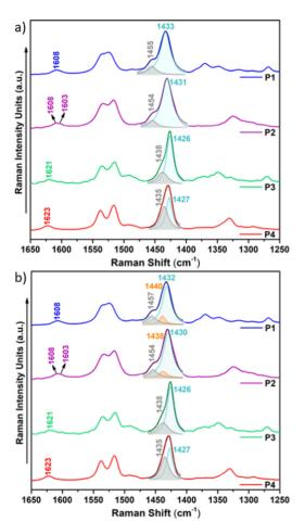
Fig. 10 Solid-state FT-Raman spectra ( $\lambda_{exc}$  = 1064 nm) of copolymers P1-P4 with (a) a simple two-component deconvolution of representative Raman bands and (b) the optimal deconvolution which best fits the experimental data
