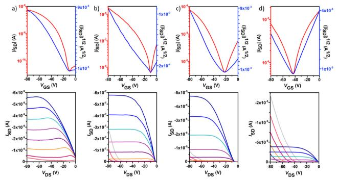
Fig. 6 Typical p-type field-effect transistor transfer (top) and output (bottom) characteristics for polymers P1 (a), P2 (b), P3 (c) and P4 (d). The transfer characteristics were measured at a source-drain voltage ( $V_{DS}$ ) of -80 V. The output curves were measured at gate voltages ( $V_G$ ) from 0 to -80 V in intervals of 10 V and over a  $V_{\rm DS}$  range of 0 to -80 V.
