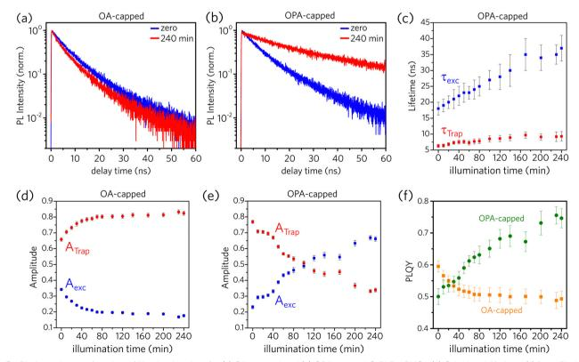
Fig. 5 PL dynamics as a function of illumination time for (a) OA-capped and (b) OPA-capped CsPbBr<sub>3</sub> PNCs. (c) Calculated lifetimes (r) from PL decay data for OPA-capped PNCs. Calculated amplitudes (A) from PL decay data for (d) OA-capped and (e) OPA-capped PNCs (Trap: trap-assisted recombination; exc: excitonic recombination). (f) Calculated photoluminescence quantum yield (PLQY) from PL decay data for OA- and OPA-capped PNCs.
