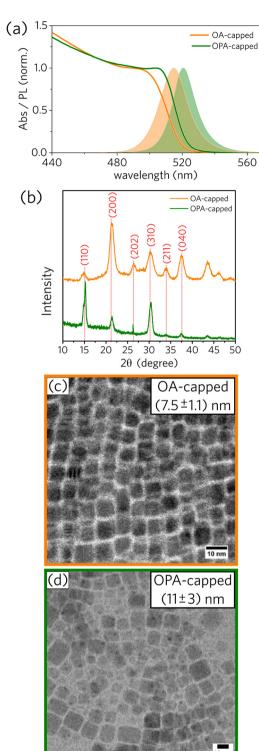
Fig. 1 (a) Absorption and PL emission spectra for OA-capped and OPAcapped CsPbBr<sub>3</sub> PNCs (OA: oleic acid, OPA: oleylphosphoric acid). (b) Diffractograms for OA-capped and OPA-capped CsPbBr<sub>3</sub> PNCs with diffraction patterns corresponding to an orthorhombic. TEM images for (c) OA- and (d) OPA-capped CsPbBr<sub>3</sub> PNCs.
