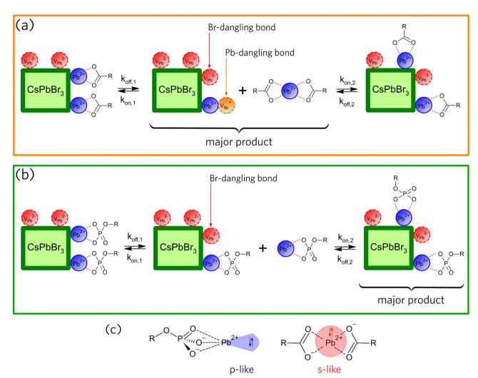
Fig. 3 Proposed mechanisms for the light-induced loss of surface components in hexane for (a) OA- and (b) OPA-capped CsPbBr<sub>3</sub> PNCs (k<sub>on</sub>adsorption rate constant;  $k_{\text{off}}$ : desorption rate constant). (c) Molecular structures of components lost from the surface during light exposure, showing the hemidirected geometry and the p-like lone-pairs for Pb(OPA), as well as the holodirected geometry and the s-like lone-pairs for Pb(OA)<sub>2</sub>.
