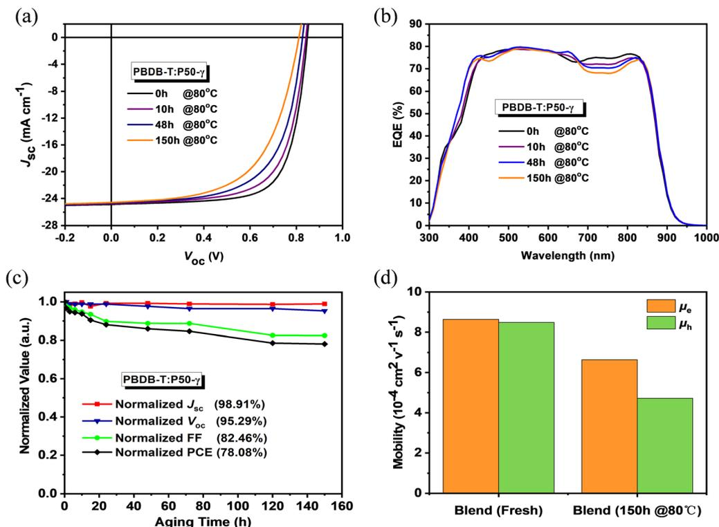
Fig. 2 (a)  $J$ - $V$  curves, (b) EQE spectra, and (c) normalized photovoltaic parameters of the PBDB-T:P50- $\gamma$ -based PSCs with different storage times under 80 °C in the  $N_2$ -filled glovebox. (d) The mobilities of the PBDB-T:P50- $\gamma$ -based devices with fresh active layer and annealed active layer at 80 °C for 150 hours.
