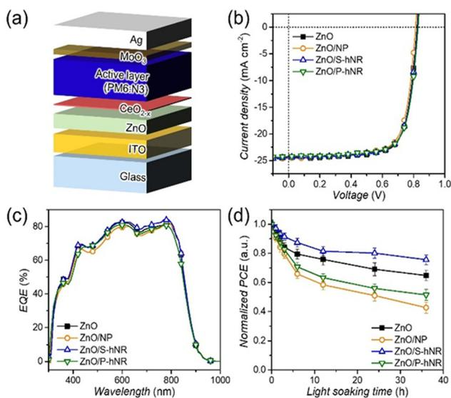
Fig. 4 (a) Schematic illustration of the OPV device. (b) *J*-*V* characteristics and (c) external quantum efficiency (EQE) spectra of the OPVs with various CeO<sub>2-x</sub>-based interlayers and (d) their dependency of normalized average PCE on light soaking time under 1 sun condition.
