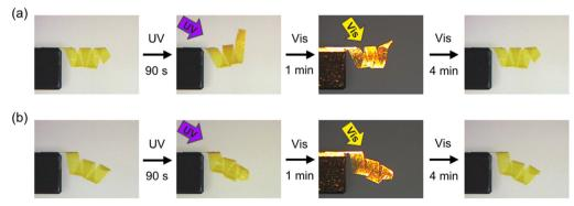
Fig. 3 Photoinduced deformation behaviors of PAzo/PMMA IPN samples with spiral shapes upon irradiation with UV (365 nm, 20 mW cm $^{-2}$ ) and visible light (>540 nm, 40 mW cm $^{-2}$ ). (a) In-plane uniaxial alignment. (b) Homeotropic alignment. Original sizes of the films: 20 mm  $\times$  1 mm  $\times$  8  $\mu$ m.
