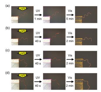
Fig. 4 Photoinduced deformation behaviours of a PAzo/PMMA IPN film with a wavy shape at (a) room temperature, (b) 100  $^{\circ}$ C, (c) 120  $^{\circ}$ C and (d) 140 °C. UV: 15 mW cm<sup>-2</sup>. Vis: 10 mW cm<sup>-2</sup>. The original size of the film: 20 mm  $\times$  1 mm  $\times$  19  $\mu$ m.
