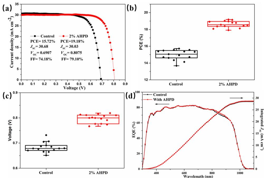
Fig. 4 (a)  $J$ - $V$  curves of the champion AHPD-treated and control devices with a reverse scan. (b) PCE distribution of the control and AHPD-treated devices. (c)  $V_{OC}$  distribution of the control and AHPD-treated devices. (d) EQE spectra of the champion AHPD-treated and control devices, and the corresponding integrated  $J_{SC}$  curves.
