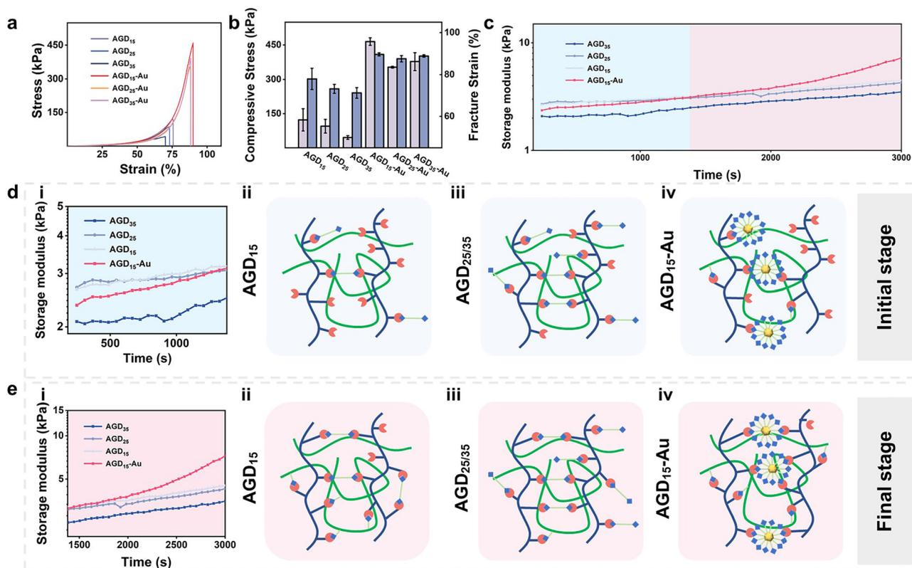
Fig. 3 (a) Compressive curves, (b) stress and fracture strain of AGD/AGD-Au hydrogels (AGD<sub>15</sub>/AGD<sub>25</sub>/AGD<sub>35</sub>/AGD<sub>15</sub>-Au/AGD<sub>25</sub>-Au/AGD<sub>35</sub>-Au), (c) the storage modulus of the prepare hydrogel vs. the time (AGD<sub>15</sub>-Au/AGD<sub>25</sub>-Au/AGD<sub>35</sub>-Au), and (d) rheological property at the initial and final stages and (i)–(iv) gelation mechanism of AGD-Au hydrogels.
