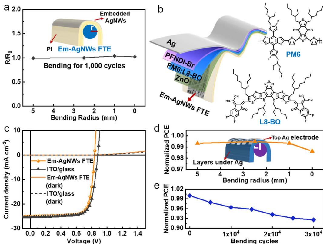
Fig. 4 Performance of the Em-AgNW FTE and related FOSC. (a) The normalized  $R_{sh}$  of the Em-AgNW FTE after 1000 bending tests at different radii. (b) Structure illustration of the FOSC and chemical structures of PM6 and L8-BO. (c)  $J$ - $V$  characteristic curves of the flexible and rigid devices. The normalized PCE values of the FOSC after 1000 bending cycles at different bending radii (d) and for cycles up to 30 000 times at a radius of 1 mm (e).
