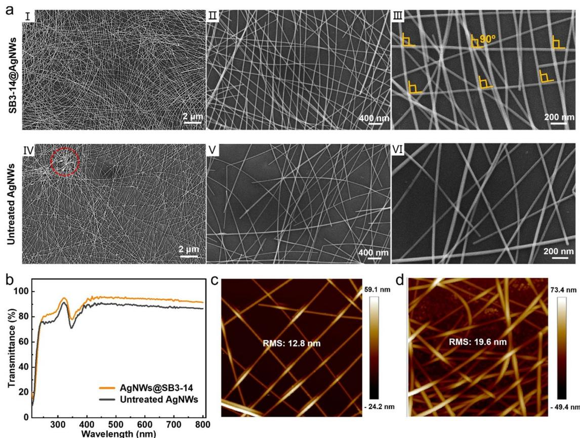
Fig. 2 Characterization of the corresponding two types of electrodes. (a) SEM images of the SB3-14@AgNW electrode (I, II and III) and the untreated AgNW electrode (IV, V and VI), where the red circle in image IV shows obvious aggregation of nanowires. (b) Optical transmittance curves. AFM height images of the SB3-14@AgNW electrode (c) and untreated AgNW electrode (d).
