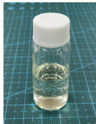
Fig. 30 Natural deep eutectic solvent-based lubricant with 100% biomass composition.
