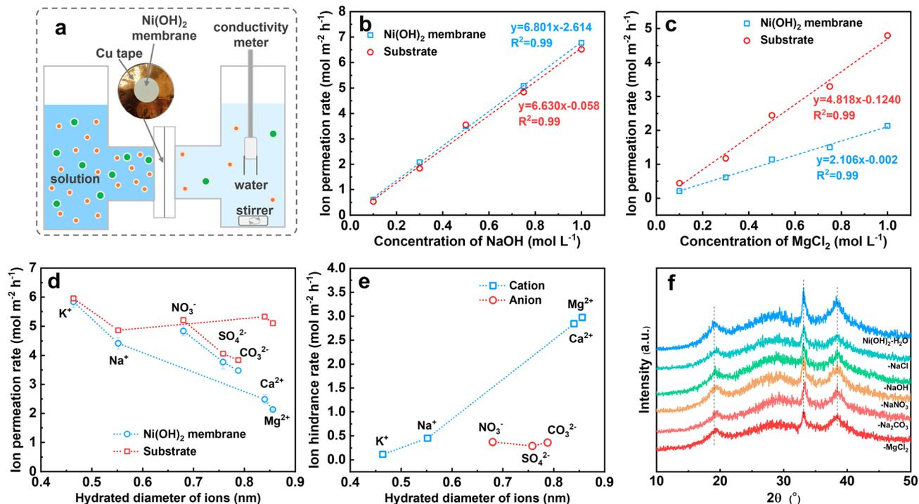
Fig. 4 (a) Schematic of Ni(OH)<sub>2</sub> membrane test setup. Ion permeation rates under different concentrations of (b) NaOH and (c) MgCl<sub>2</sub> solutions. (d) Ion permeation rate versus ion hydrated diameter of the substrate and Ni(OH)<sub>2</sub>-membrane-coated substrate. (e) The calculated ion hindrance rate for the Ni(OH)<sub>2</sub> membrane. (f) XRD patterns of Ni(OH)<sub>2</sub> membrane powder after immersion in different solutions.
