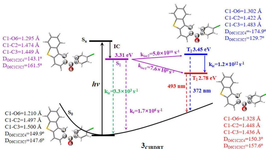
Fig. 3 The adiabatic energy levels, radiative ( $k_r$ ) and nonradiative ( $k_{\text{ic}}$  and  $k_{\text{isc}}$ ) rates, as well as T<sub>1</sub> and T<sub>2</sub> emission wavelengths for  $3_{\text{CIBDBT}}$ . The ground state energy (-1660.75414666 a.u.) of  $3_{\text{CIBDBT}}$  is set as the reference at the CC2/cc-pVDZ level. The geometrical parameters for some important bonds and dihedral angles are also shown.
