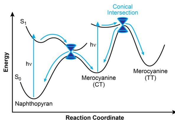
Fig. 3 Representative reaction pathway for the photochemical ring-opening reaction of naphthopyran.
