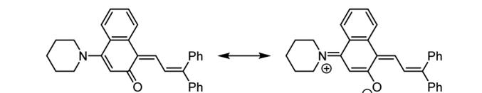
**Scheme 12** Amine substituents can stabilize *3H*-naphthopyran-derived merocyanines through resonance.
