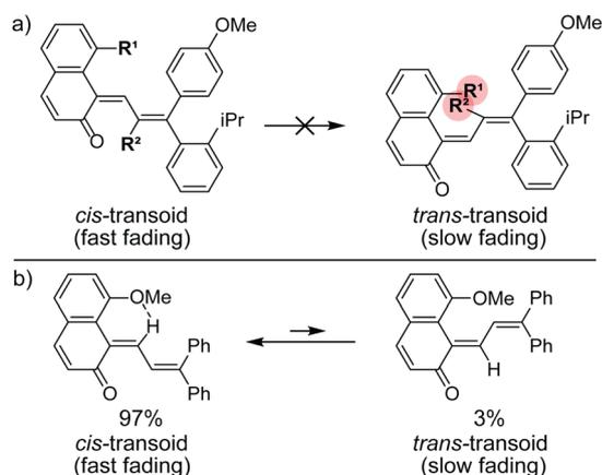
Scheme 13 (a) Substituents at the 2- and 10-positions of 3*H*-naphthopyrans result in severe steric repulsion in the *trans* merocyanine. (b) Hydrogen bond acceptors at the 10-position of 3*H*-naphthopyrans stabilize the *cis* merocyanine stereoisomer.
