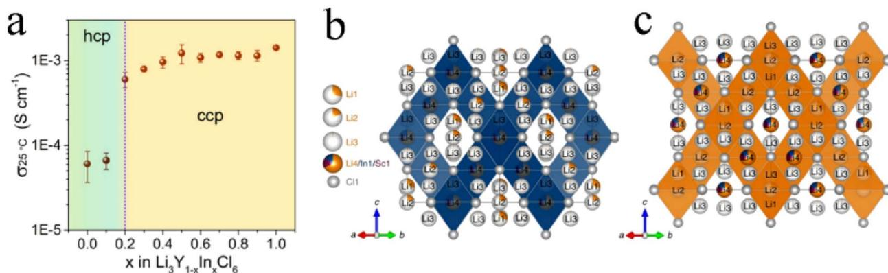
Fig. 6 (a) Ionic conductivity of  $\text{Li}_3\text{Y}_{1-x}\text{In}_x\text{Cl}_6$  with different In contents at 25 °C. Reproduced with permission.<sup>38</sup> Copyright 2020, American Chemical Society. Structure (b) and the main 3D Li ion diffusion pathway (c) of  $\text{Li}_2\text{In}_{1/3}\text{Sc}_{1/3}\text{Cl}_4$ . Reproduced with permission.<sup>46</sup> Copyright 2022, Springer Nature.
