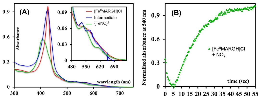
Fig. 5 (A) Intermediate absorption spectrum (blue) upon addition of  $[\text{NBu}_4]\text{NO}_2$  to  $[\text{Fe}^{\text{II}}\text{MARGH}]\text{Cl}$  (red) and the corresponding final spectrum of  $\{\text{FeNO}\}^7$  species (green). (B) Kinetic trace followed at 540 nm for the formation of  $\{\text{FeNO}\}^7$  complex upon addition of 100 equivalents of  $[\text{NBu}_4]\text{NO}_2$  to  $[\text{Fe}^{\text{II}}\text{MARGH}]\text{Cl}$ .
