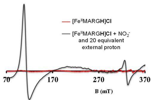
Fig. 8 X-band EPR spectra of  $[\text{Fe}^{\text{II}}\text{MARGH}]\text{Cl}$  (red) upon simultaneous addition of 5 equivalents of  $[\text{NBu}_4]\text{NO}_2$  and 20 equivalents of 2,6-xylylidinium chloride (dark grey).
