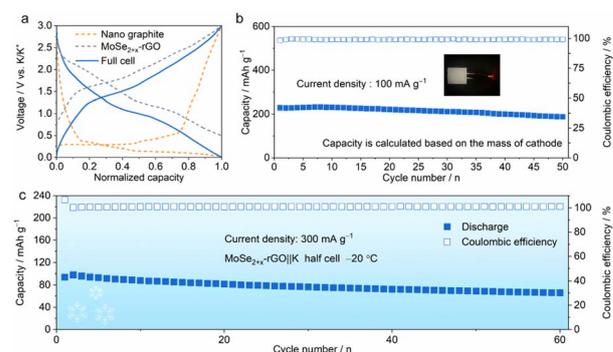
Fig. 5 Electrochemical performance of the MoSe<sub>2+x</sub>-rGO||NG full cell and MoSe<sub>2+x</sub>-rGO||K half cell at low temperature. (a) Discharge/charge profiles of the half cell and the full cell. (b) Cycling performance of the MoSe<sub>2+x</sub>-rGO||NG full cell at 100 mA g<sup>-1</sup>; the inset is a corresponding optical image showing it powering a LED. (c) Cycling performance of the MoSe<sub>2+x</sub>-rGO||K half cell at 300 mA g<sup>-1</sup> and -20 °C.
