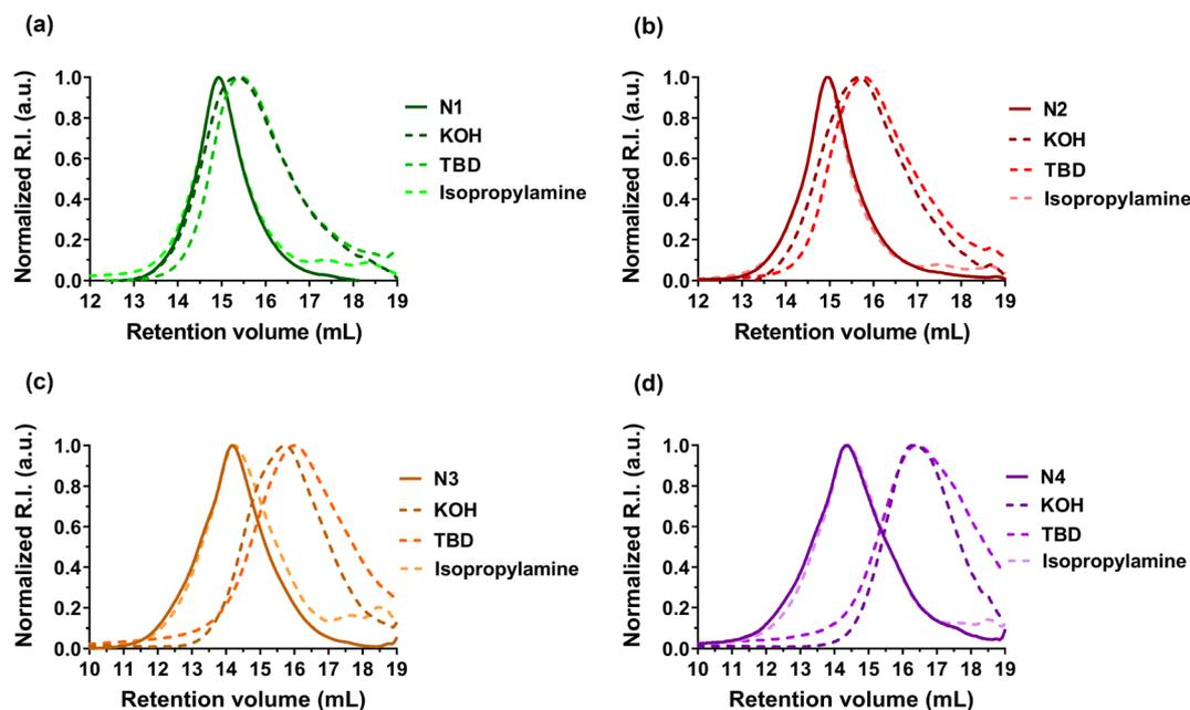
Fig. 4 Evolution of the SEC chromatograms of P(I-co-DOT) copolymers: (a) **N1**, (b) **N2**, (c) **N3**, and (d) **N4**, after degradation under basic (KOH or TBD) or aminolytic (isopropylamine) conditions.
