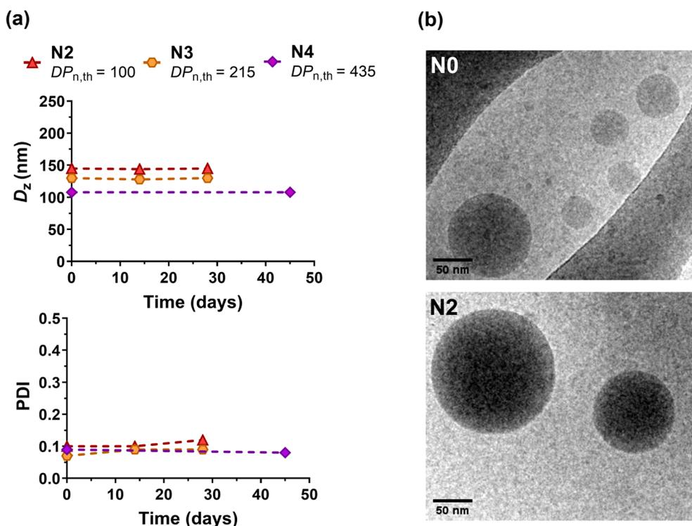
**Fig. 5** (a) Evolution of the intensity-average diameter ( $D_z$ ) and polydispersity index (PDI) with time measured by DLS of P(I-co-DOT) nanoparticles (N2, N3 and N4, Table 3). (b) Representative cryo-TEM images of nanoparticles N0 and N2.
