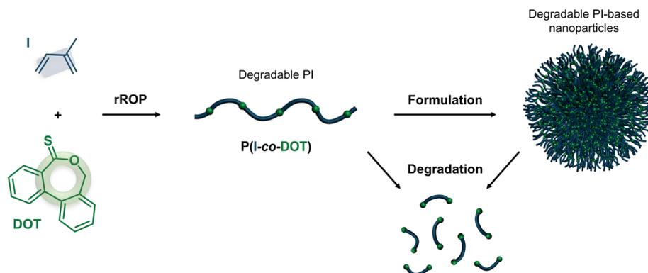
Fig. 1 Synthesis of degradable vinyl polymer nanoparticles *via* radical ring opening copolymerization (rROP) of dibenzoc[*c,e*]oxepane-5-thione (DOT) and isoprene (I) in solution followed by nanoprecipitation.
