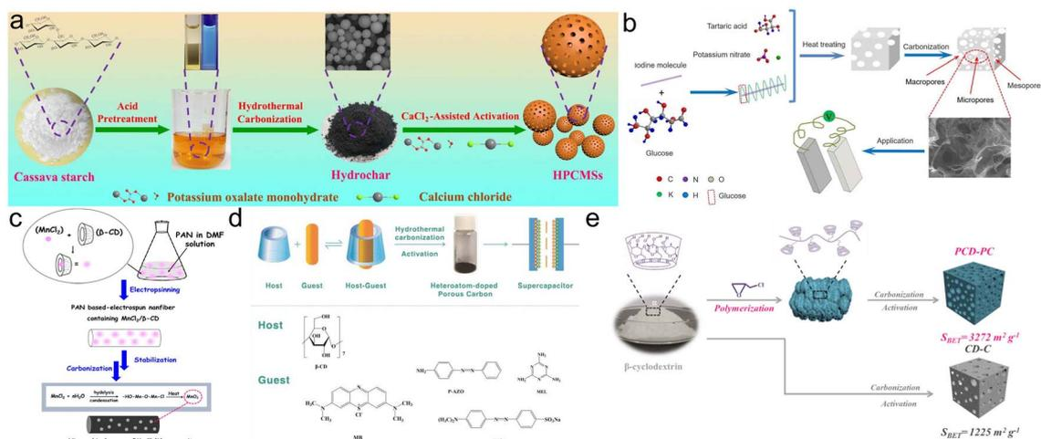
Fig. 6 (a) Illustration for the synthesis of HPCMSs;<sup>64</sup> (b) scheme for the preparation of I-PCs-X;<sup>66</sup> (c) diagram for the construction of PMnCD( $\beta$ );<sup>67</sup> (d) schematic for the preparation mechanism of porous CMs;<sup>68</sup> (e) mechanism diagram for the synthesis of the PCD-PC.<sup>69</sup>
