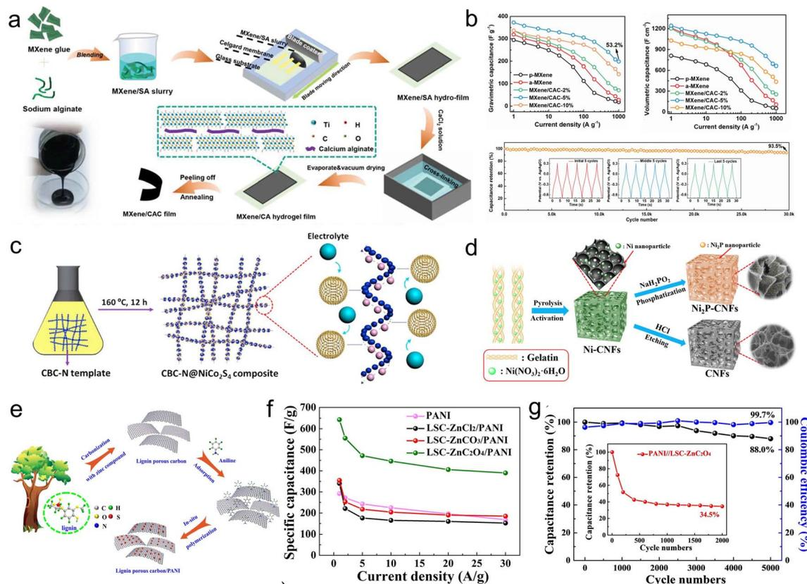
Fig. 12 (a) Scheme for the synthesis of MXene/CAC films; (b) capacity and cycling stability test of MXene/CAC;<sup>150</sup> (c) scheme for the space-confined growth of CBC-N@NiCo<sub>2</sub>S<sub>4</sub> composite;<sup>155</sup> (d) diagrams for the preparation of Ni-CNFs, Ni<sub>2</sub>P-CNFs and CNFs;<sup>156</sup> (e) schematic for the fabrication of lignin porous carbon/PANI composites; (f) specific capacitance of the samples; (g) cycling test of LSC-ZnO/PANI//LSC-ZnO ASCs.<sup>161</sup>
