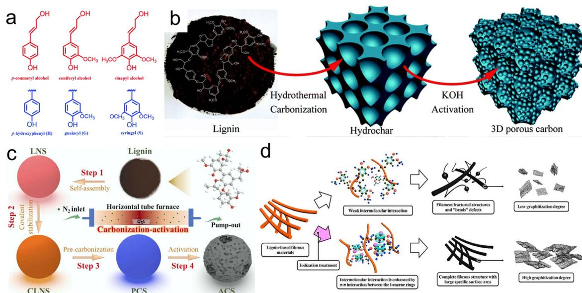
Fig. 4 (a) Monomer units and precursors of lignin;<sup>49</sup> (b) illustration for the fabrication of LHC;<sup>52</sup> (c) diagram for the synthesis of ACS-600;<sup>53</sup> (d) structure comparison between carbon fibers by iodization and original carbon fibers.<sup>55</sup>
