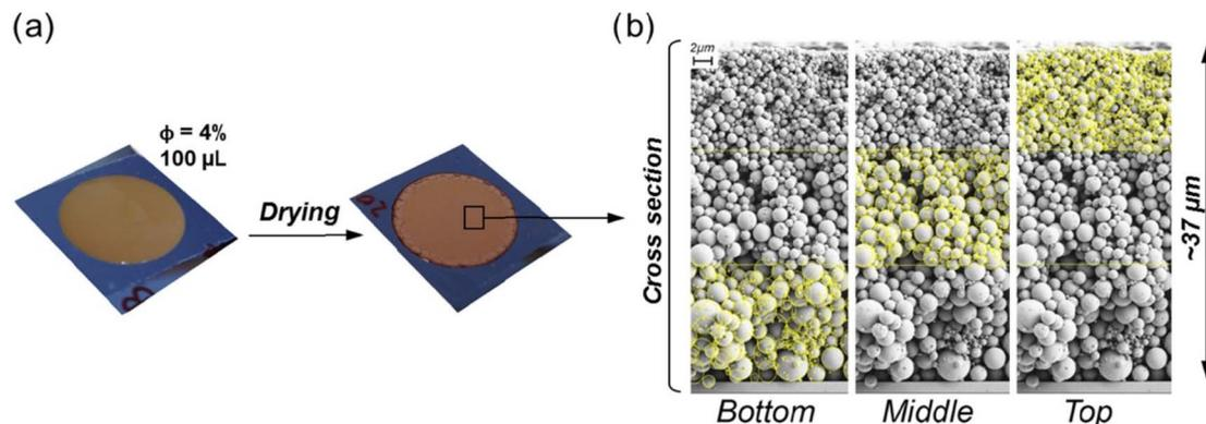
Fig. 8 Coatings comprising lignin particles produced by evaporation-induced self-assembly (a) and vertical cross-section of the obtained layers (b).<sup>85</sup>
