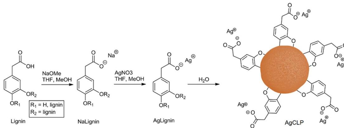
Fig. 12 Simplified schematic of the production of silver-doped lignin nanoparticles.<sup>129</sup>
