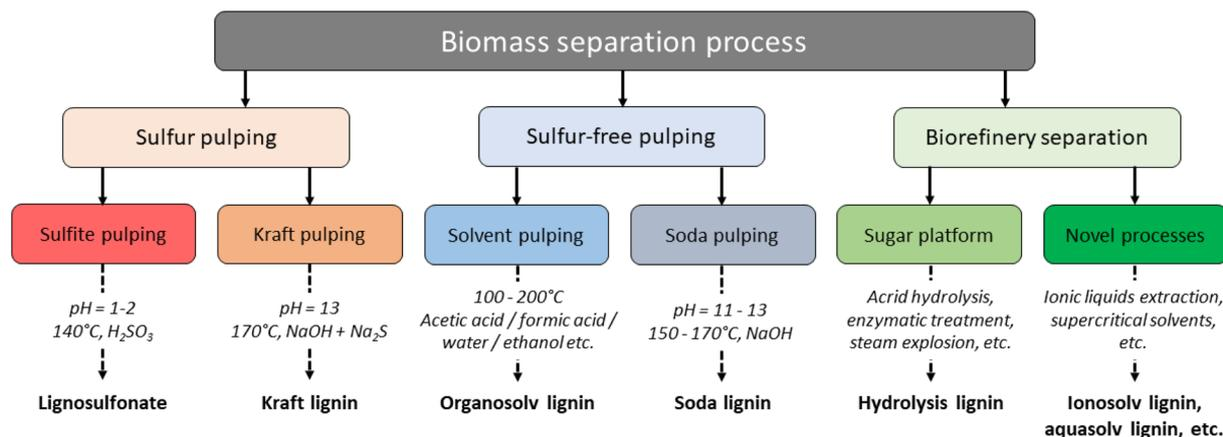
Fig. 5 Lignin extraction processes and their products.<sup>3</sup>
