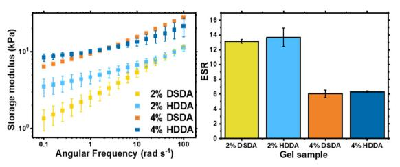
Fig. 2 Characterisation of PBA-DSDA and PBA-HDDA networks: shear storage modulus, G', of as-synthesised gel discs by oscillatory rheology (left) and ESR of gel samples in THF (right).
