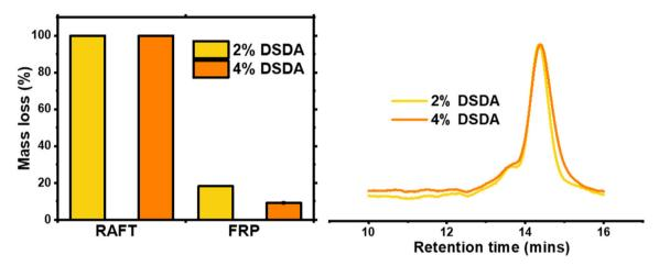
Fig. 3 Degradation of PBA-DSDA gels by 25 mg  $mL^{-1}$  DTT solution in DMF. Left: Mass loss % referenced to original mass of dry gel sample before degradation. 100% mass loss corresponds to macroscopic degradation of gel to soluble fragments. Right: GPC traces of soluble fragments from fully degraded PBA-DSDA RAFT networks.
