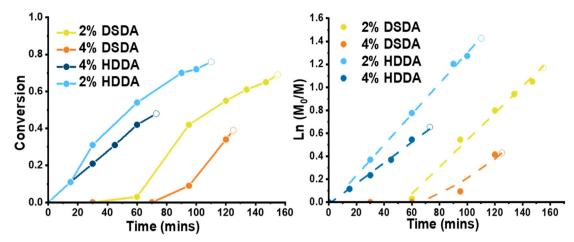
Fig. 1 Conversion plots (left) and first-order semi-logarithmic kinetic plots (right) for RAFT polymerisations of PBA-DSDA and PBA-HDDA networks. The final point on each data set (open symbol) is the estimated acrylate conversion at the gel point from gel times and through linear regression of the kinetic plots. [BA]: [DDMAT]: [AIBN]: [X] = 100:1:0.2:2 or 4, X = DSDA or HDDA. BA: anisole 1:1 v/v; 65 °C, 24 h.
