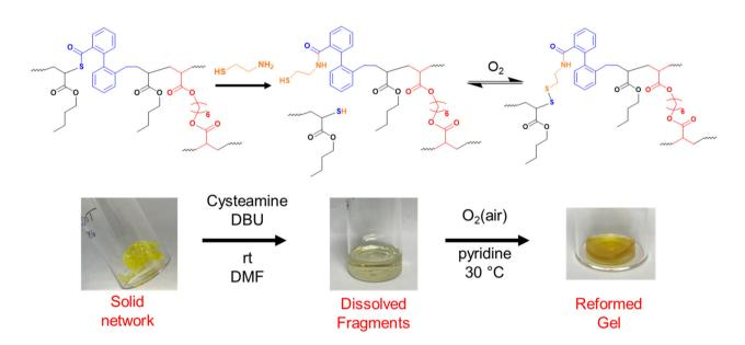
Fig. 8 Degradation and regelation scheme for PBA-DOT networks. Images of PBA-DOT3 sample.
