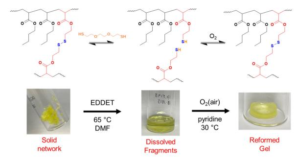
Fig. 7 Degradation and regelation scheme for PBA-DSDA networks. Images of PBA-DSDA5 sample.
