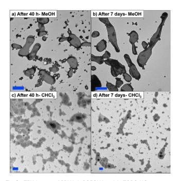
Fig. 8 TEM images of PBMA-b-POEGMA vesicle TORC-NGs as conversion of CBMA increases showing large, elliptical polymersomes at low conversions (a) that transition to large, multi-micron long tubesome structures at full CBMA conversion (b). The stability of these materials at both stages is confirmed upon solvent switch to CHCl<sub>3</sub> and imaging using TEM (c, d; all scale bars =  $2.0 \mu m$ ).
