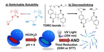
Fig. 1 Multi-responsive TORC-NG materials, synthesized in one-pot via PhotoATR-PISA, which can fully disassemble only when first exposed to acidic aqueous environments (pH = 4; a) followed by UV-C irradiation () = 254 nm) and thiol reducing agents (b).
