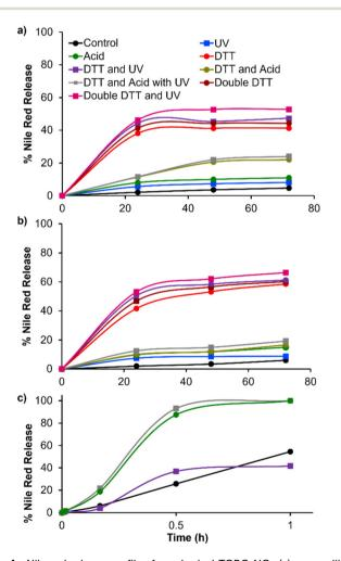
Fig. 4 Nile red release profiles for spherical TORC-NGs (a), worm-like TORC-NGs (b) and non-CCL nanosphere (c) upon application of various stimuli simultaneously (legend applies to all plots; control = no stimuli; acid = adjusted to pH 4 with HCl/H<sub>2</sub>O; DTT = addition of 66.2 mM DTT for spherical TORC-NG and 51.1 mM DTT for worm-like TORC-NG; UV = 1 h irradiation with 254 nm UV light).
