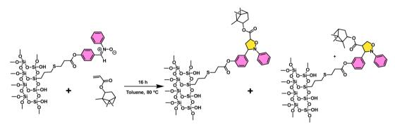
Scheme 5 1,3-Dipolar cycloaddition of nitrone functionalized RHA silica with isobornyl acrylate.
