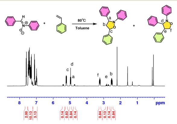
Fig. 5 <sup>1</sup>H NMR spectrum of the cycloadduct formed from styrene and *N*-1-diphenylmethanimine oxide and the peaks present at  $\delta$  = 2.5 ppm-3.5 ppm and 4.5 ppm-5.5 ppm confirms the formation of the cycloadduct.
